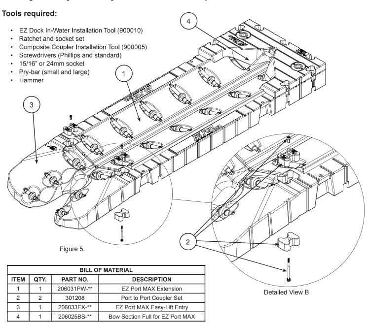
**NOTE:** Testing has also shown that some watercrafts and user preference resulted to water ballasting the entry (206033EX-\*\*) with water (see EZ Launch Owners Manual). This is done by simply filling the entry with water to the desire level. This allows the watercraft an easier entry and even a more stable platform.
